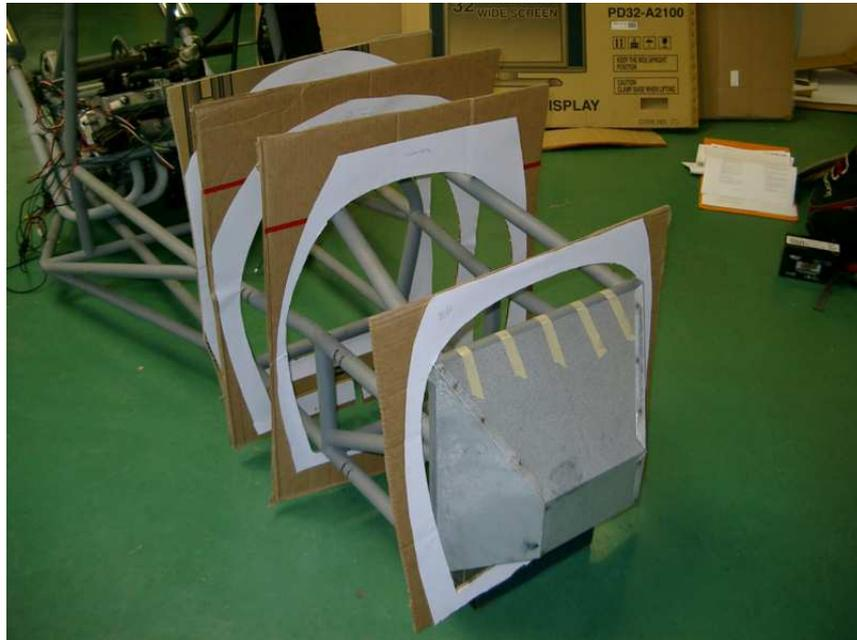
Figure 6.14: Checking nosecone fit with cardboard sections
