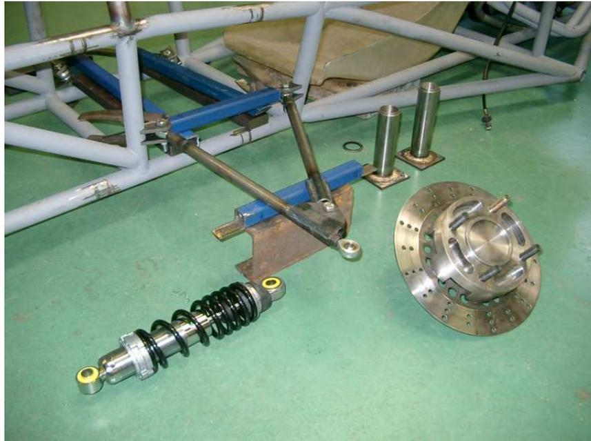
Figure 6.9: Modified front suspension under construction
