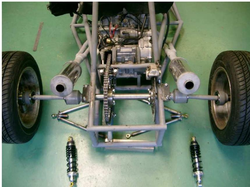
Figure 6.7: Rear suspension under construction
