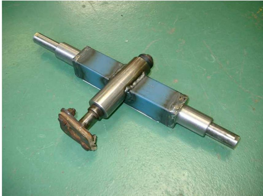
Figure 6.5: The modified steering rack during construction
