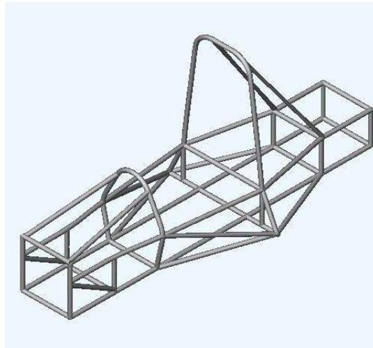
Figure 6.1: Solid model of the chassis
