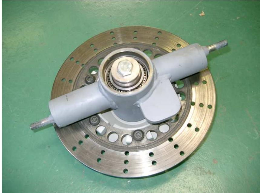
Figure 6.6: Front upright, hub and rotor assembly prior to modification
