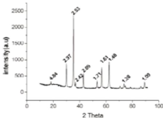
Fig. 1: X-ray diffraction of MNPs.
